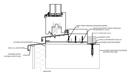
INNOVA SLIDING DOOR THRESHOLD NEEDS TO BE SUPPORTED UNDERNEATH TO AVOID BENDING
